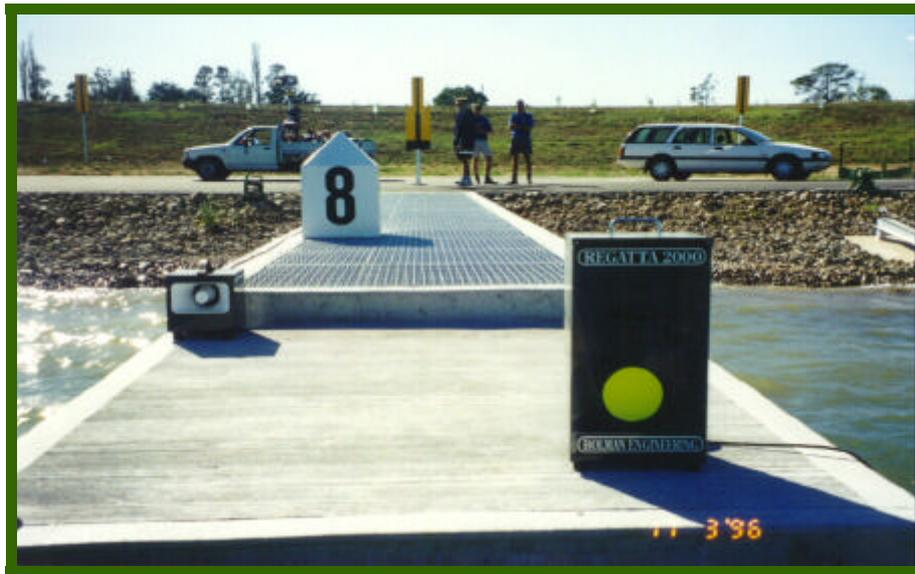
The start signal is generated by the Start Console by either pressing a button, or by firing a starting gun (the start gun signal is picked up automatically). Below is a photo of the start console.
