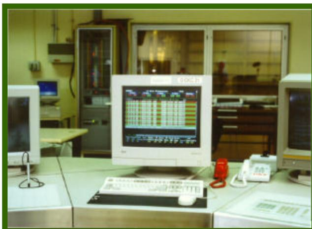
The photo left shows one of the screens for the man/machine interface. Holman Engineering's user friendly software enables the operator to use either the keyboard or the mouse to carry out all functions.
